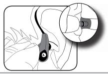
To change earphone sleeve, twist and pull sleeve to remove it from the nozzle. Push new sleeve onto nozzle until you feel it slide completely over barb. If any part of the nozzle is exposed, sleeve is not properly installed. Replace sleeves if they do not grip the nozzle tightly
